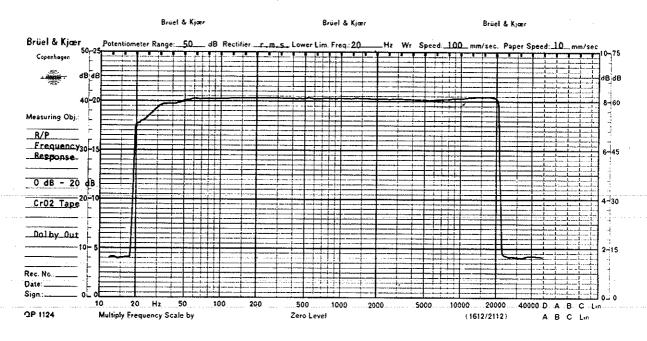
Fig.18 Record/Playback Frequency Response (Dolby NR Out)
