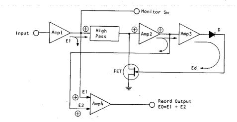
Fig.3 Record Dolby Processor System Diagram
