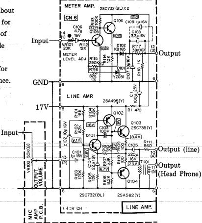
Fig.21 Meter & Line Amp. P.C.B. Circuit Diagram
