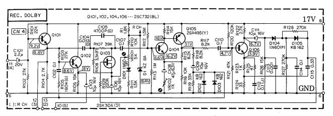
Fig.1 Record Dolby Processor Circuit Diagram
