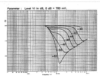
Fig.9 Dynamic Noise Limiter Steady-State Characteristics
