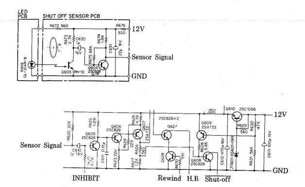
Shut-off Sensor and Detector Circuit Diagram
