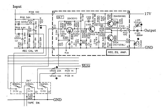
Fig.16 Rec. EQ. Amp. Circuit Diagram
