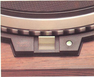
The LED strobe is precisely controlled by the crystal oscillator circuit.
